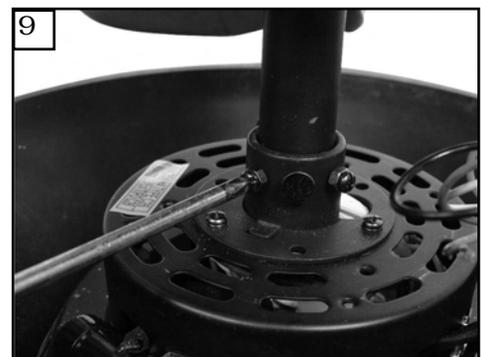
Tighten 2 downrod set screws and lock nuts.
