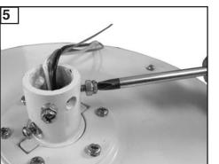
Loosen the 2 set screws and nuts till you can not feel them on inside of yoke.
