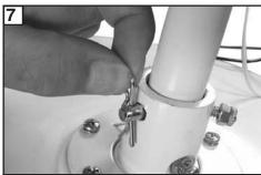
Insert downrod into yoke on top of fan body. Align the hole in the downrod with hole in the yoke. Insert pin through the yoke and downrod until the point appears on the other side. Install the keeper.
