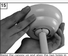
Raise the canopy up and align the two holes in the canopy with the two holes in the hanger bracket. Twist into place. Secure with two screws provided.
