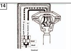
For control of fan and optional light from wall location, follow diagram above. NOTE: A professional electrician is recommended for this type of installation.
