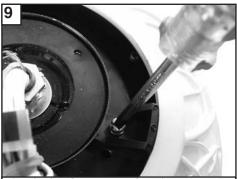
Check the fan motor for shipping stabilizer and remove if present.
