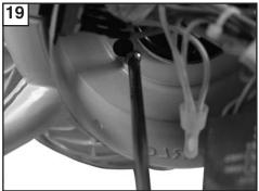
Install switch plate by placing over the 2 screws and twisting into place. Install screw removed and tighten all 3 screws securely.
