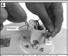
Remove keeper from pin. Pull pin out and replace keeper, save for later.
