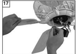
Check the motor for shipping stabilizer and remove if present. Attach blade assembly to motor using the motor screws and washers provided. Tighten screws securely.
