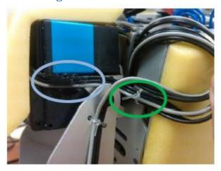
In order to protect the servo wires from unnecessary abrasion during routine usage, we suggest using some kind of rubber glue or silicone adhesive on the wire.
