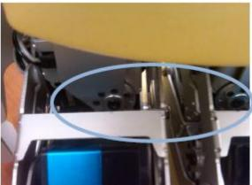
When configuring the robot stand from the sitting position, or to sit from the standing position, assure that the servo horns are behind the forward part of the upper leg bracket, in order to prevent damage to the servo and frame. This must be done manually when the power to the servo is turned OFF when configuring the robot while in the seated position.
