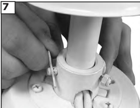
**7** Insert downrod into yoke on top of the Fan Body. Align the hole in the Downrod with the hole in the Yoke. Insert the Pin through the Yoke and Downrod until the point appears on the other side. Install the keeper to pin.
