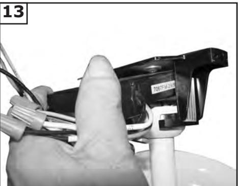
**13** Slide remote receiver into mounting bracket.
