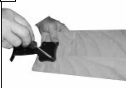
Place blade arms onto the other side of the blade and aligning holes. Insert screws with fabric washers through the holes and tighten securely.
