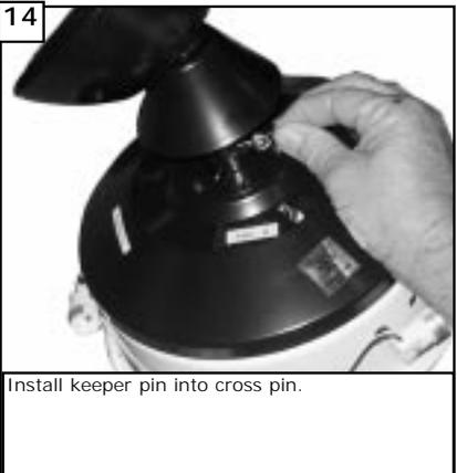
Install keeper pin into cross pin.
