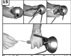
Install Canopy Cover, Cage Assembly and Yoke cover onto the Downrod. Next thread the fan leadwire from top of fan through the downrod.
