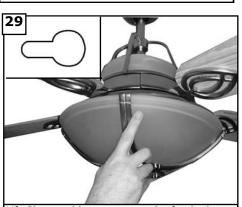
Lift Glass and lower cage to the fan body. Align the 4 screws on the cage with 4 keyhole slots in fan body (See Inset for keyhole shape. Rotate the glass and cage counter clockwise to lock into place.
