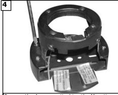
Remove the 4 screws attaching the Mounting neck the mounting plate. Retain the 4 screws for re-assembly.
