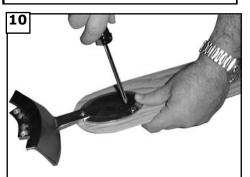
Place the Main holder over the blade and install 3 screws and tighten securely. Repeat this process again for each blade
