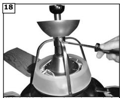
Slide the Yoke Cover, and cage down on the fan body. The Cage should engage 4 slots in the upper glass. Tighten the Set Screw in on the top of the Cage. This will prevent any rattling.
