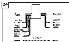
Make wiring connections as indicated above. White from fan to white from remote marked N. Orange from fan to Orange from remote marked Light/up. Blue from fan to blue from remote marked down light. Black from fan to Red from remote marked L. White from house to white from remote marked AC N. Black from house to Black from remote marked AC L. Connect all green ground wires to Ground wire from House.
