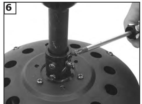
**6** Tighten the 2 Set screws on the Yoke once the downrod is in place.
