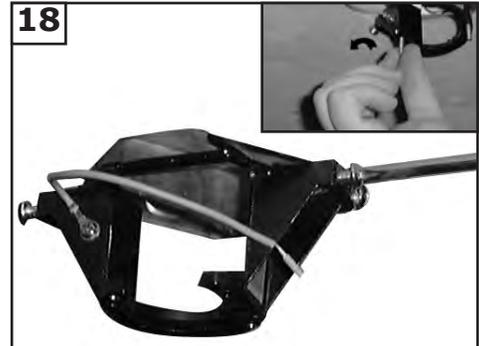
18 Take 4 screws from hardware pack and insert 2 one on each side of bracket to match the L slot screw holes in canopy. Keep 2 screws for later use. Remove the all thread studs from the lower part of the mounting bracket.
