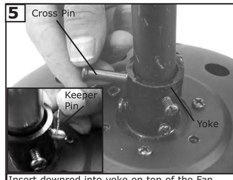
**5** Insert downrod into yoke on top of the Fan Body. Align the hole in the Downrod with the hole in the Yoke. Insert the Pin through the Yoke and Downrod until the point appears on the other side. Install the Keeper Pin
