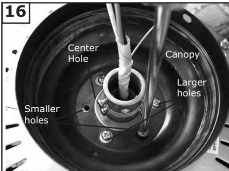
16 Place canopy on top of the fan motor allowing the yoke to pass through the large hole in the center of the canopy. Align the 3 larger holes around the center hole with the 3 screws already installed in the fan. Install 3 flush mount screws provided into smaller holes and tighten securely.
