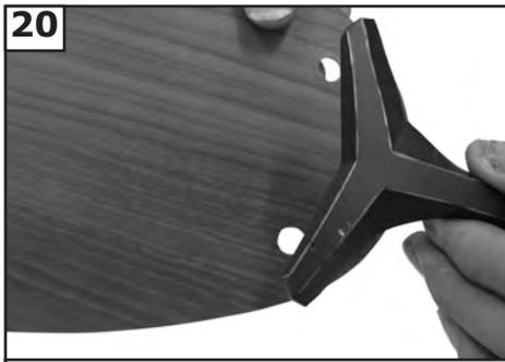
Place blade holders onto blades aligning holes in blade holder with holes in blade. Make sure that the side of the blade you select is facing downward. Install 3 screws and fiber washers to back side of blade as shown. Tighten screws securely. Repeat this process 3 more times until all blades are assembled.
