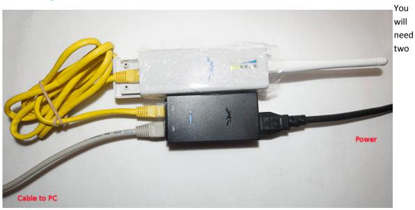
Ethernet cables (Cat-5) that are not supplied with the unit.
