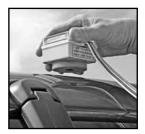
Step 1 The transmitter is equipped with a magnetic base. When placing the transmitter on the tow vehicle, always locate the most secure position possible.
