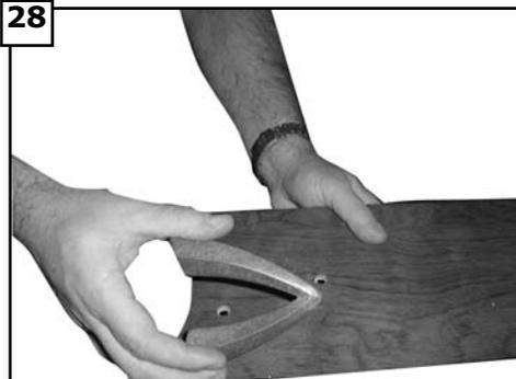
28 Place floating brackets onto blades aligning holes in blade with the floating bracket.
