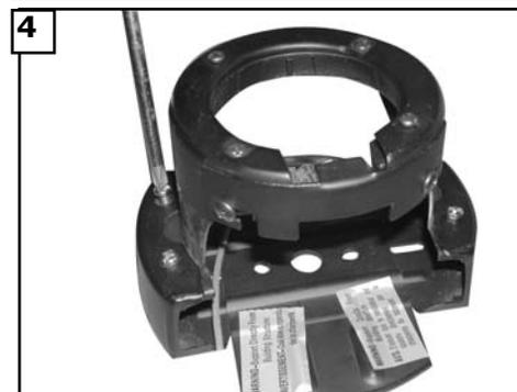
4 Remove the 4 screws attaching the Mounting neck the mounting plate. Retain the 4 screws for re-assembly.
