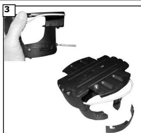
3 Remove Safety bar from mounting bracket by loosening screws, sliding bar to side, and lifting it off the 2 screws.
