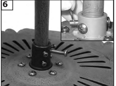
Insert downrod into motor yoke. Next, insert clevis pin through yoke and downrod and secure with cotter pin. (see inset)
