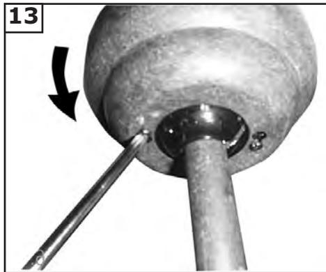
Raise the canopy up and align the two holes in the canopy with the two holes in the hanger bracket. Secure with two screws provided.
