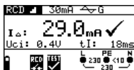
Figure 5.20: Example of trip-out current measurement result
