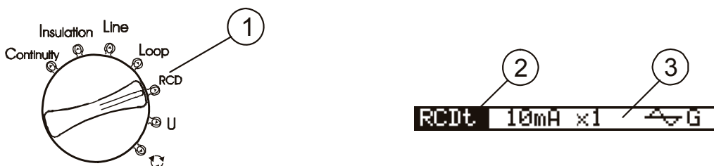
Figure 4.2: Function selector switch and belonging parameter line
