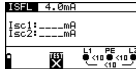
Figure B.4: First fault current measurement menu
