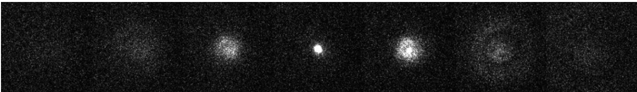
Illustration 29: Fluorescent bead imaged at 1000nm intervals. The central frame is in focus. Contrast levels have been set to show the PSF when out-of-focus.
