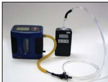
Adjust flow with flow adjust screw on tube holder.
