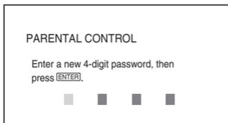
Enter a 4-digit password using the number buttons, then press ENTER. The display for confirming the password appears.
