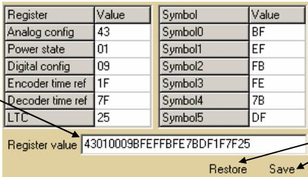
Registers configuration of the MLX90121 transceiver. Start from address 0 (AnalogConfig register) to address 11 (LTC register)
