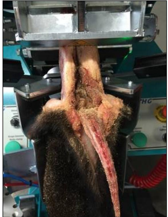
**4.** The leg clamp is now shut, let the animal hang loose in the leg clamp, (Left pedal is still held down) grab the tail skin from the animal, while the second hand pushes the tail clamp over the animal, while the tail skin is put in the clamp, the clamp closes automatic when it is pushed over the animal (watch out that our fingers do not get the clamp). The tail from the body may not get in the clamp.
