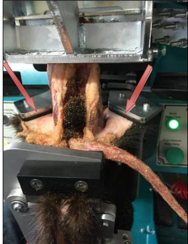
**6.** Adjusting when the slow pull is activated is done by moving the sensor on the side of the body cover. The sensor is activated when Leg clamp runs up past the sensor. The sensor makes the machine pull slowly and support clamp for the skin closes, and the leg skin clamp opens
