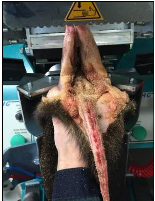
**3.** The leg clamp is closed by pressing the left pedal and holding it down.
