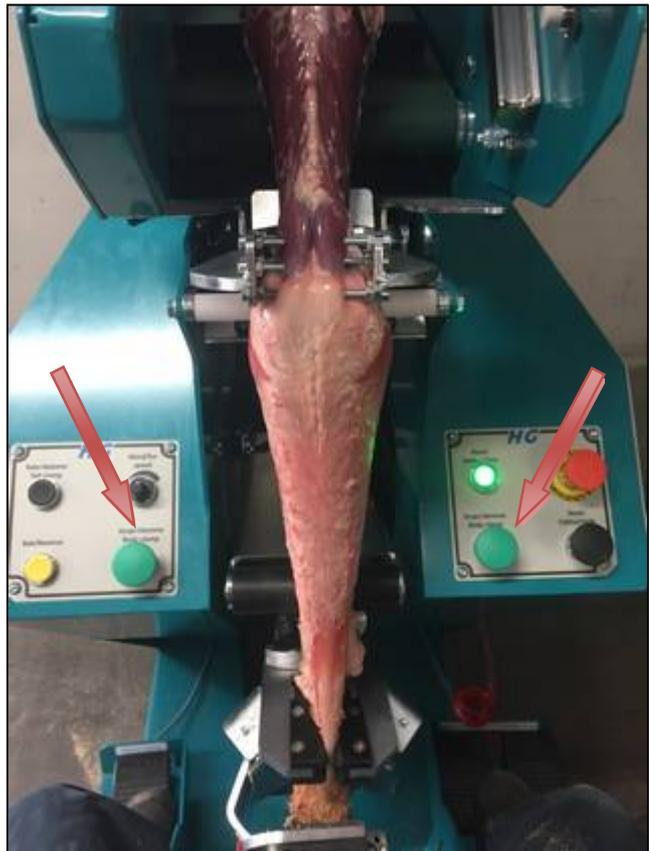
**10.** Continue pressing on the pedal for fur pull until the skin is pulled down over the shoulders to the head.
