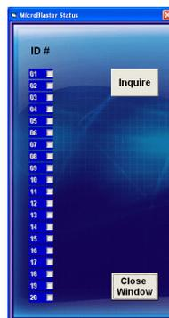
Push the “Inquire” button and wait for the test to be complete. If the microblaster is plugged in and working properly, the checkbox in this screen will be checked.
