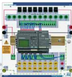
PLC Board 24 V with KNX extension module
