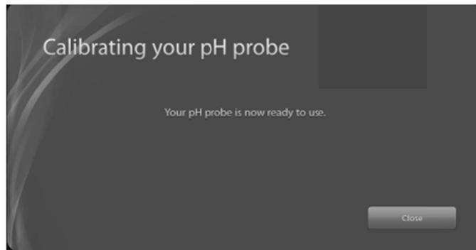
When the pH Calibration wizard displays ‘Your pH probe is now ready to use,’ remove the pH probe from the calibration solution and rinse the probe in RODI water. Then press or click on the ‘Close’ button in the Calibration wizard. The pH calibration process is now complete and your pH probe is ready to be installed in your tank.
