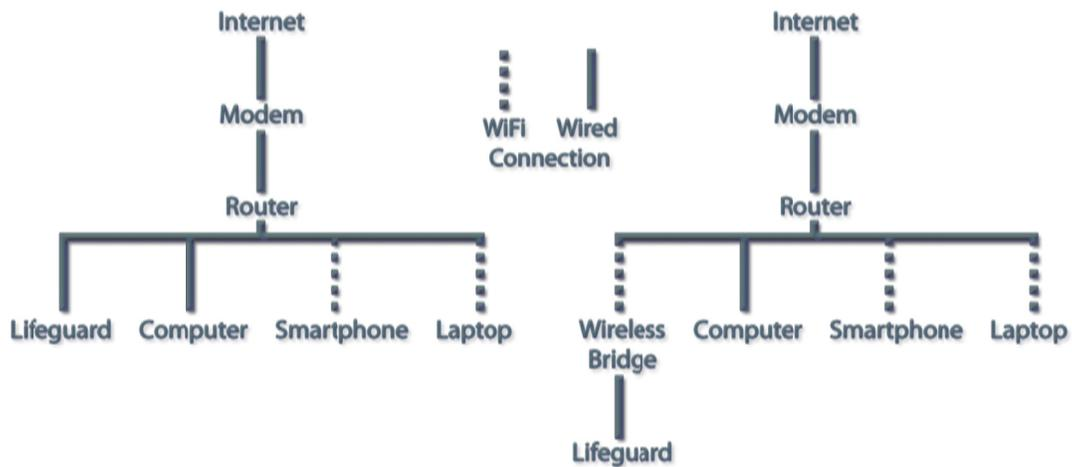
Routers are designed to stop unauthorized access from over the Internet. To access Lifeguard from the Internet, you'll need to configure your router to enable *port forwarding*, also known as *port mapping*. Port forwarding allows an external, internet-connected computer or device to communicate with computers or devices (such as Lifeguard) in your home or office network.
