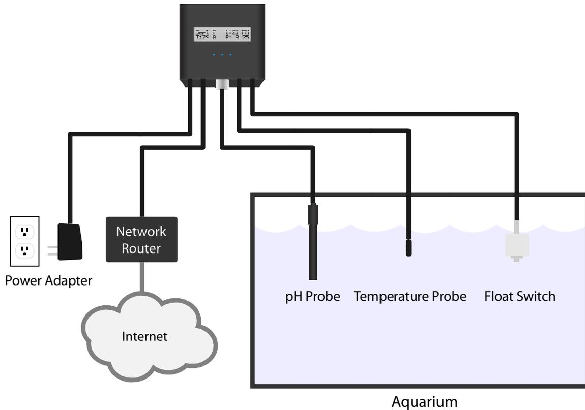
*Lifeguard monitoring system – typical installation*
