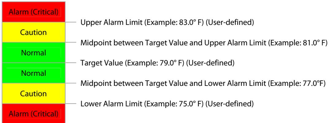
Caution conditions are triggered when temperature or pH values cross the midpoint between the target value and the high or low alarm value.
