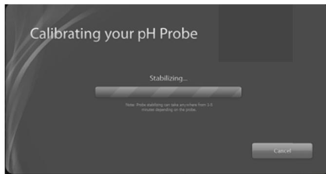
When the pH probe is adequately stabilized, press or click on the 'Start' button. The pH Calibration wizard screen will report 'Stabilizing...' and display a barber pole indicator while the calibration is in progress. The calibration process may take several minutes.
