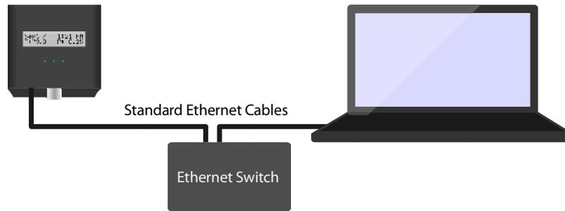
**Connection diagram via Ethernet switch**
