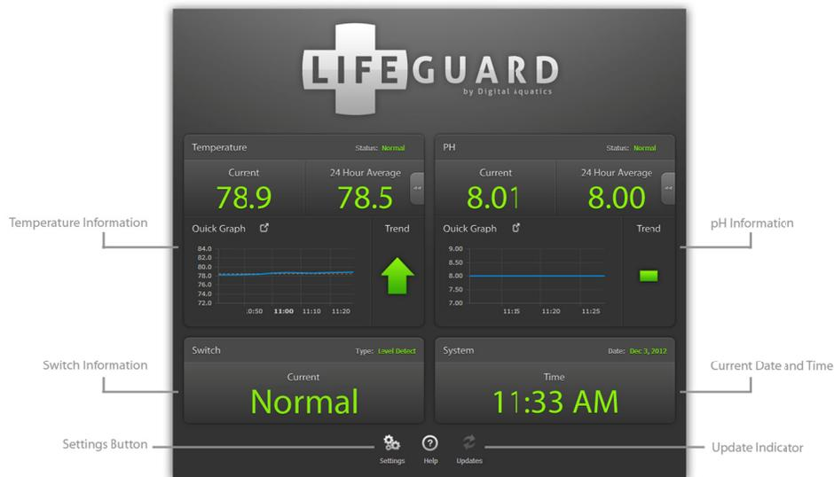
The Lifeguard web server's dashboard displays current and 24-hour average readings, graphing and trend information for both pH and temperature inputs. The dashboard also displays the switch input status as well as the current date and time. The dashboard also provides a Settings button that links to the settings menus, a Help button (which accesses this guide) and an Update indicator/button that enables access to Lifeguard firmware updates.
