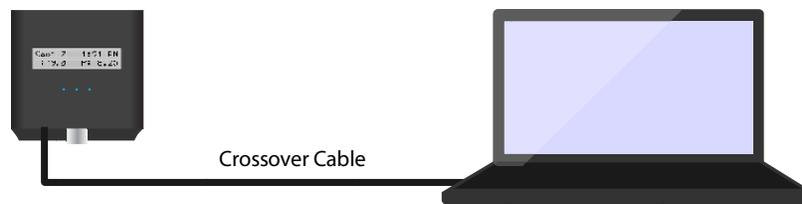
**Connection diagram via Ethernet crossover cable**
