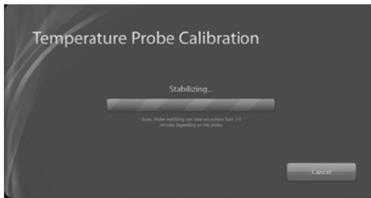
The Temperature Calibration wizard screen will report 'Stabilizing... ' and display a barber pole indicator while the calibration is in progress. Calibration may take a few minutes.
