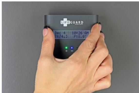
Digital Aquatics recommends mounting Lifeguard vertically. It is important that your electronic equipment never be mounted on the ground or in the bottom of a cabinet where water can pool. Lifeguard is best mounted as high above a level surface as conditions will allow.
