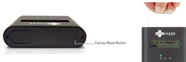
**Resetting Lifeguard with a paperclip**
