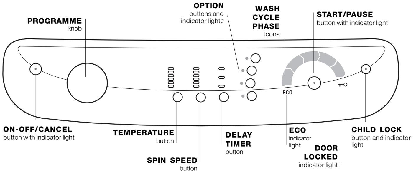
**ON-OFF/CANCEL** button with indicator light : press the button briefly to switch the machine on or off. The green indicator light shows that the machine is switched on. To switch the washing machine off during a wash cycle, press and hold the button for approximately 2 seconds; pressing the button quickly or accidentally will not switch the machine off. If the machine is switched off during a wash cycle, the programme will be cancelled.
