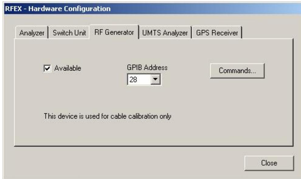
Any suitable RF generator with a GPIB interface can be used. The optionally available tracking generator of a GPIB controlled spectrum analyzer (FSP, FSU or ESPI) can be used as well.
