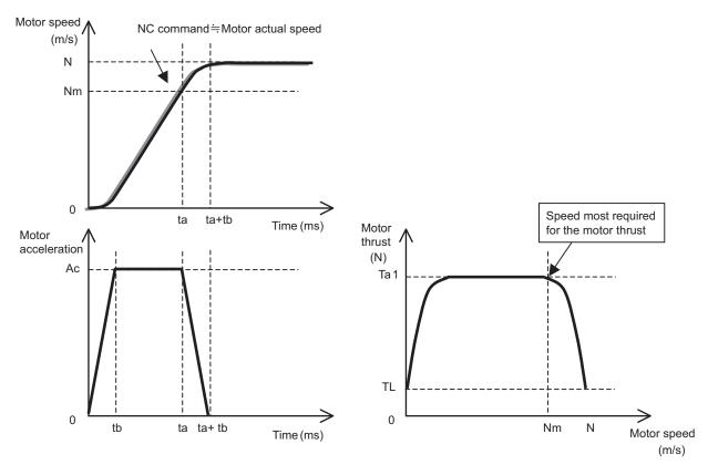
Fig 3. Speed, acceleration and thrust characteristic when using the NC command soft acceleration/deceleration pattern + feed forward (high-speed accuracy) control
