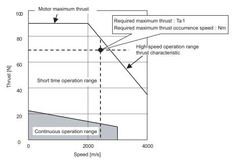
Motor thrust characteristics
