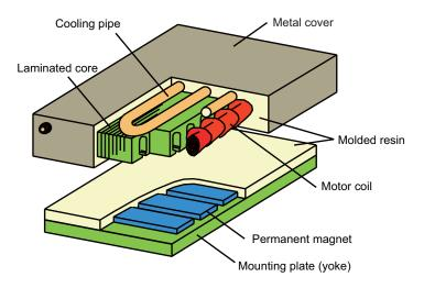
Fig. 1 Structure of linear servo motor
