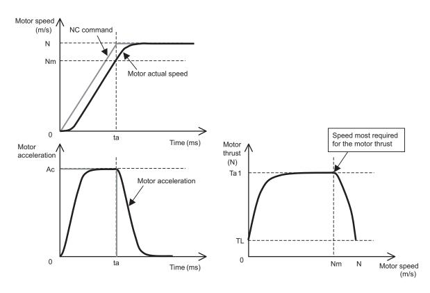
Fig.2 Speed, acceleration and thrust characteristics when using the NC command linear acceleration/deceleration pattern + servo SHG control
