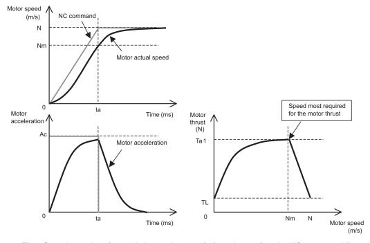
Fig.1 Speed, acceleration and thrust characteristics when using the NC command linear acceleration/deceleration pattern + servo standard position control
