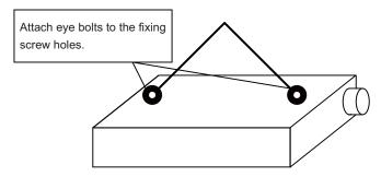
We recommend that you attach the primary side (coil) to the slider and then attach the hanging tools to the slider before suspending the primary side.
