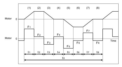
Fig. 5-1Continuous operation pattern
