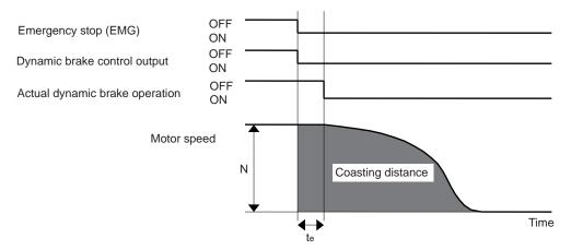
Dynamic brake braking diagram
