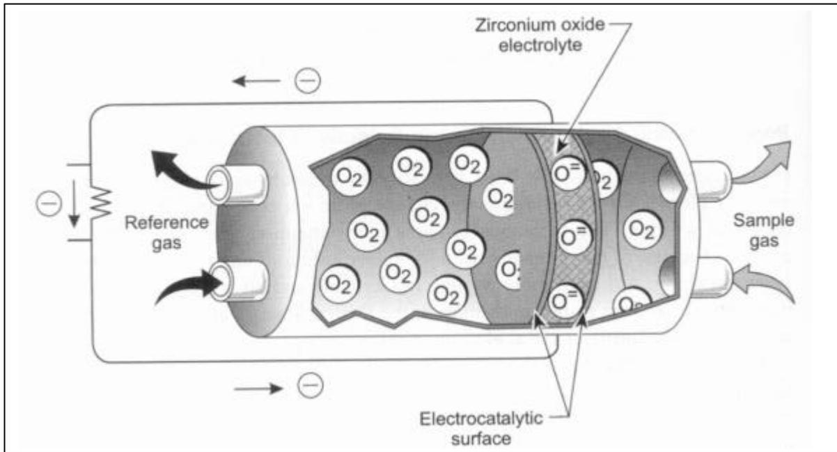
The electro-motive force (emf) that is generated across the solid electrolyte by the passage of oxygen ions, can be measured as a sensor voltage.
