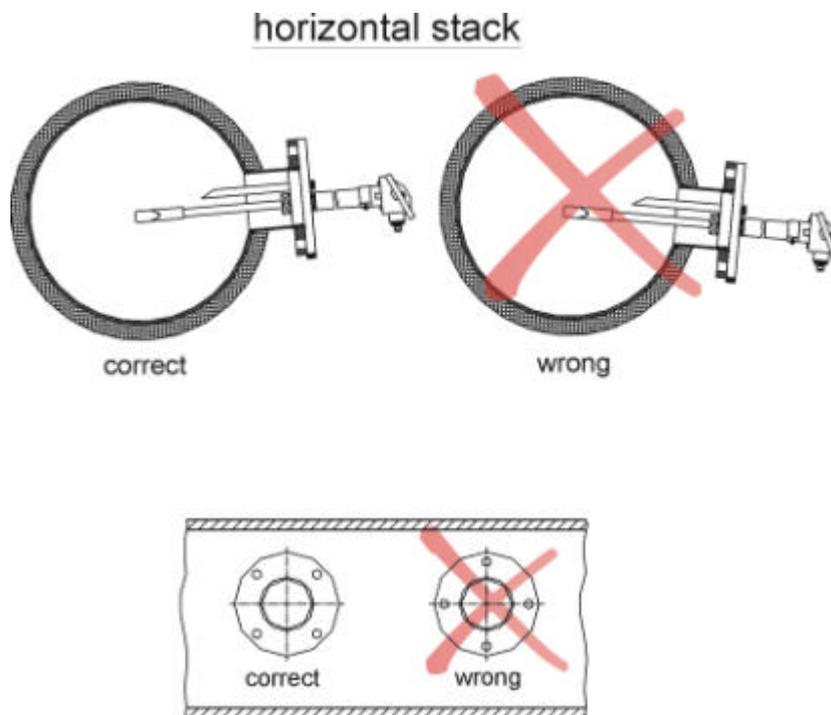
Clean the surface of the tube and drill a hole with a diameter of 110 mm into the exhaust channel. Fix the tube with few welding points, adjust it correctly and weld it completely to the steel skin of the stack.
