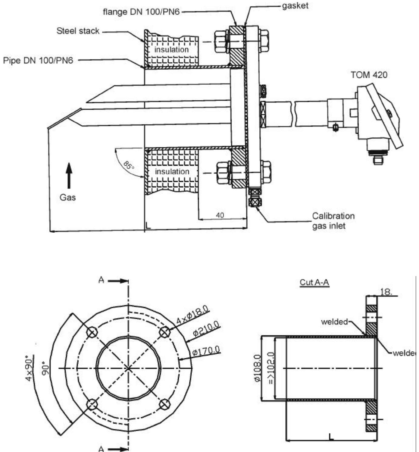
illustration pipe/flange assembly (supplied by customer)
