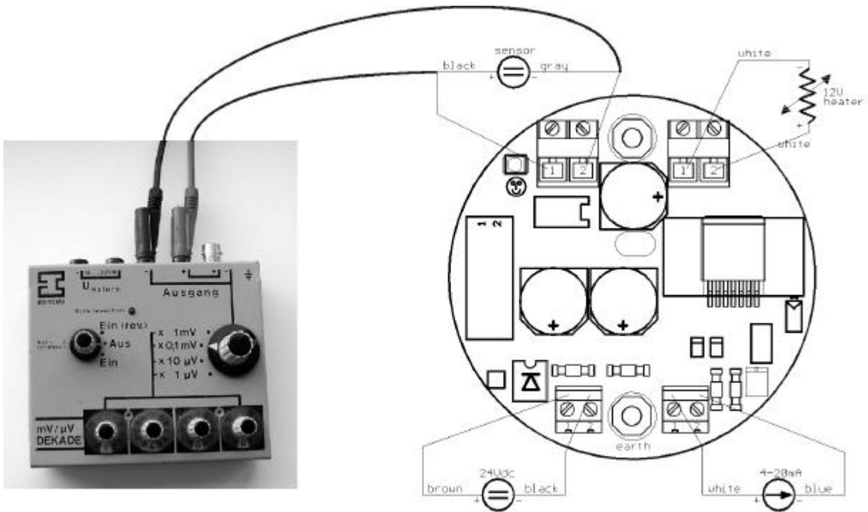
Connect precision voltage source in place of sensor signal input.
