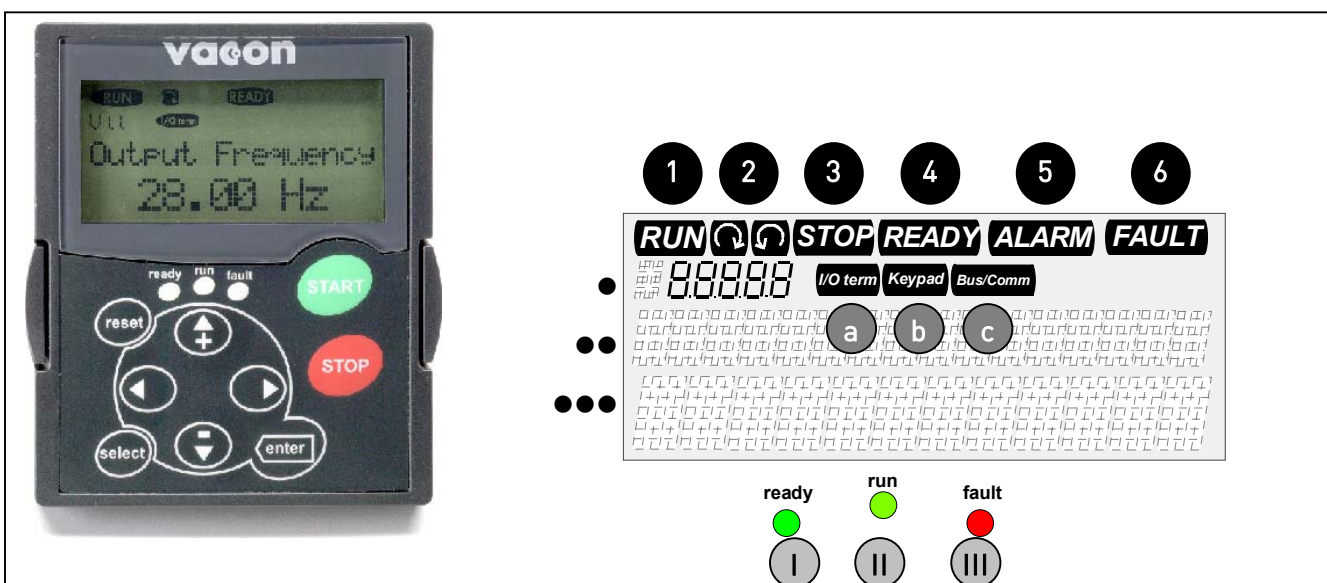
Figure 7-1. Vacon control keypad and drive status indications
