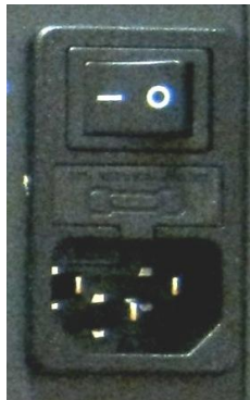
IEC Mains Socket, fuse holder and switch
