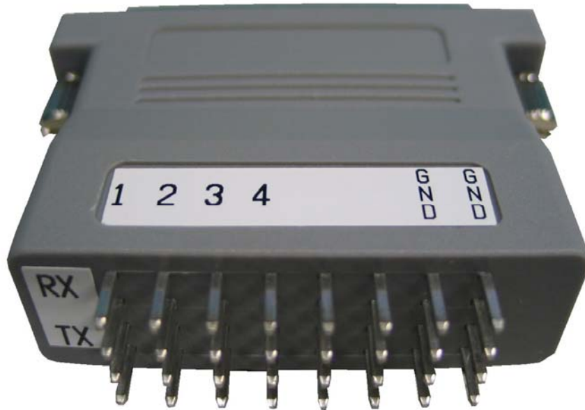
Figure 3-3 DB37 to Wire-Wrap Adapter for 4E1/T1 Port
