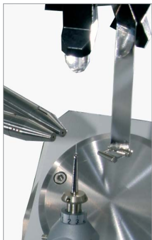
SuperNova dual wavelength beam stop with focusing LED illumination
