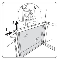
To replace the glass panels obey the procedure in opposite sequence. Before you lower the trim attach the A trim part to the door. Refer to picture.
