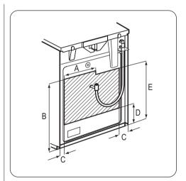
/ Warning! The gas bayonet must be in mark area.
