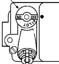
NOTE: Knob can not be turned from "PILOT" to "OFF" unless knob is pushed in slightly. Do not force.
