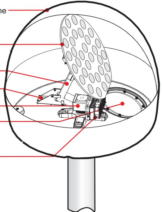
Figure 3 Antenna parts - mast mounted version.
