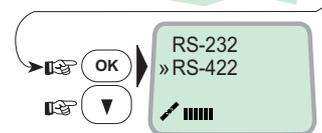
The **RS-422** is now activated for connection of e.g. PC using cables of up to 100 m.
