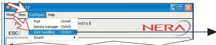
Clicking **Configure > Print handling** opens the **Printout from modem** window. The following settings are selectable:
