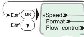
**4** Select listed **format**: 8 data bits, no parity and 1 stop bit (default)
