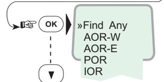
*The antenna performs an hemispheric search at antenna elevation angles varying within 0° through 90°.*
