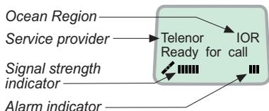
The alarm indicator flashes when an alarm condition occurs. The indicator stops once the alarm has been read in the Display Handset by pressing **MENU > Information > Alarms & messages**".
