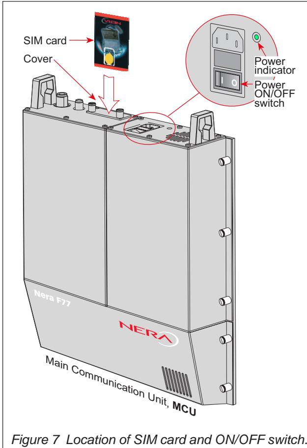
Figure 7 Location of SIM card and ON/OFF switch.
