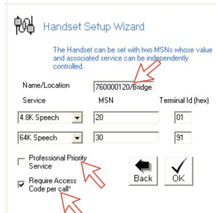
**Require Access Code** must be unchecked to allow this Handset to be used without entering a code. **Professional Priority Service** is checked on special agreement with the Net Provider, e.g. for higher priority in the Inmarsat system.
