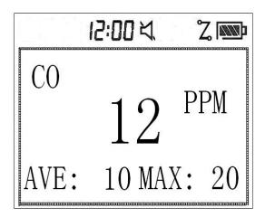
The top of the LCD shows the time, battery capacity and other signs at real time, such as the alarm status, buzzer status and link status of the communication.
