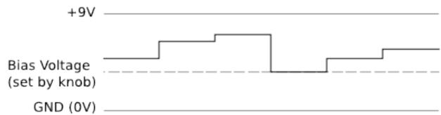
CV Signal inside the pedal
