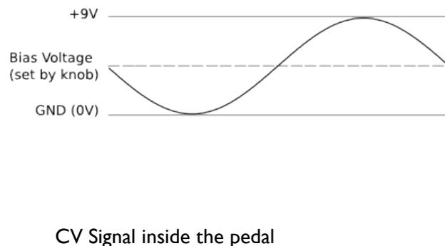
So, what happens? The incoming CV signal is shifted around the voltage that you select with the corresponding knob. Example: if you insert a -5V to +5V sine wave into the RESONANCE CV jack you will
