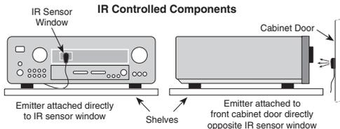
> Peel off the adhesive cover and affix the emitter to the center of the IR sensor window on the controlled component's front panel
