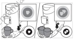
11 When the water has heated up and the on/ off button lights up continuously, the machine starts brewing coffee.
