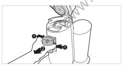
**5** To disassemble the coffee spout, grab the two ridges of the inner part of the spout and squeeze them lightly (1). Move the inner part downwards to remove it from the outer part of the spout (2).
