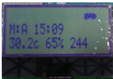
Figure 13 LCD display when slave device is in Sensor Logger Mode
