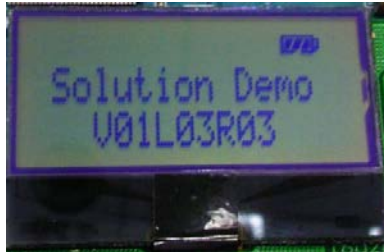
Figure 11 LCD display when host device or slave device is in Remote Control Mode
