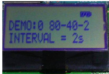
Figure 12 LCD display when host device is in Sensor Logger Mode
