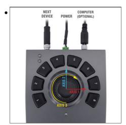
Default axes are setup with X as 1, Y as 2 and Z as 3
