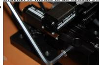
Slide bracket over optical post into desired position and tighten M6 screw with 5 mm allen key to lock M-LSM in position.
