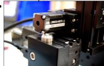
Ensure that the optical post doesn't extend too far, or it will interfere. The above image shows incorrect installation where the optical post will obstruct the movement.
