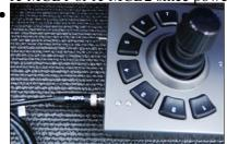
The X-JOY3 is connected to the X-MCB2 through the X-DC06 cable
