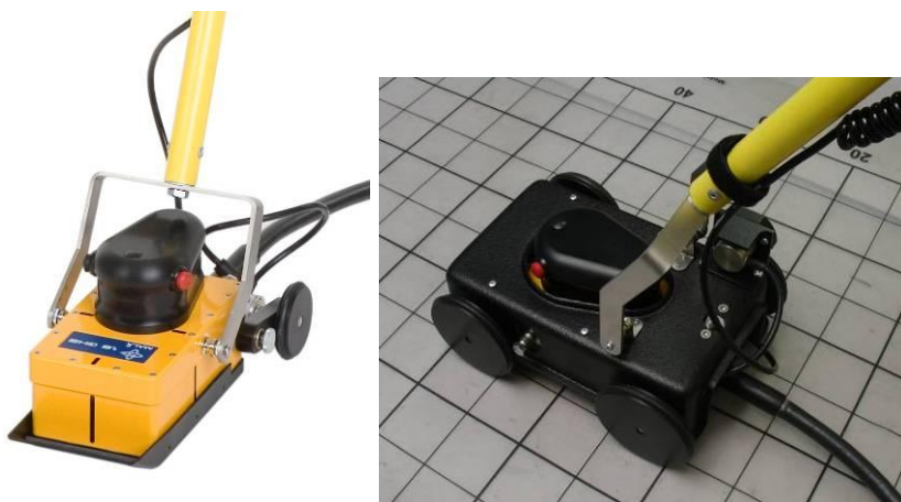
Figure 12.7 Mounting of the extension handle.
