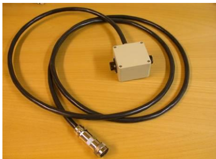
Figure 12.8. Switch box for two High Frequency antennas.
