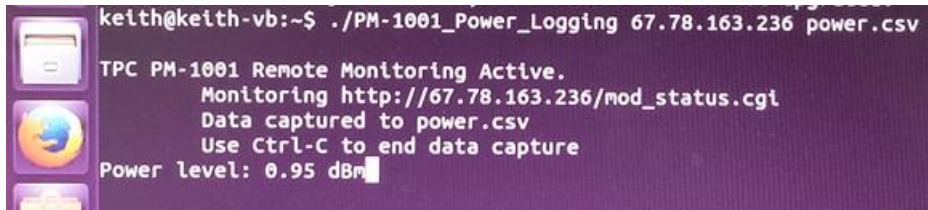
Figure 7.5.1-1 – Linux Computer’s Display Once Data Logging Has Begun
