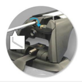
Tighten adjusting screw to 5 Nm.
