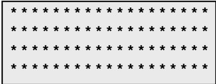
Press DO three times. You should see a full screen of "8", then full screen of "=", and finally a full screen of "I". If any of the screens do not display correctly, then something is wrong with the display of the TDC-12. Contact us using the information in the front of this manual to arrange to ship the TDC-12 back for repair.
