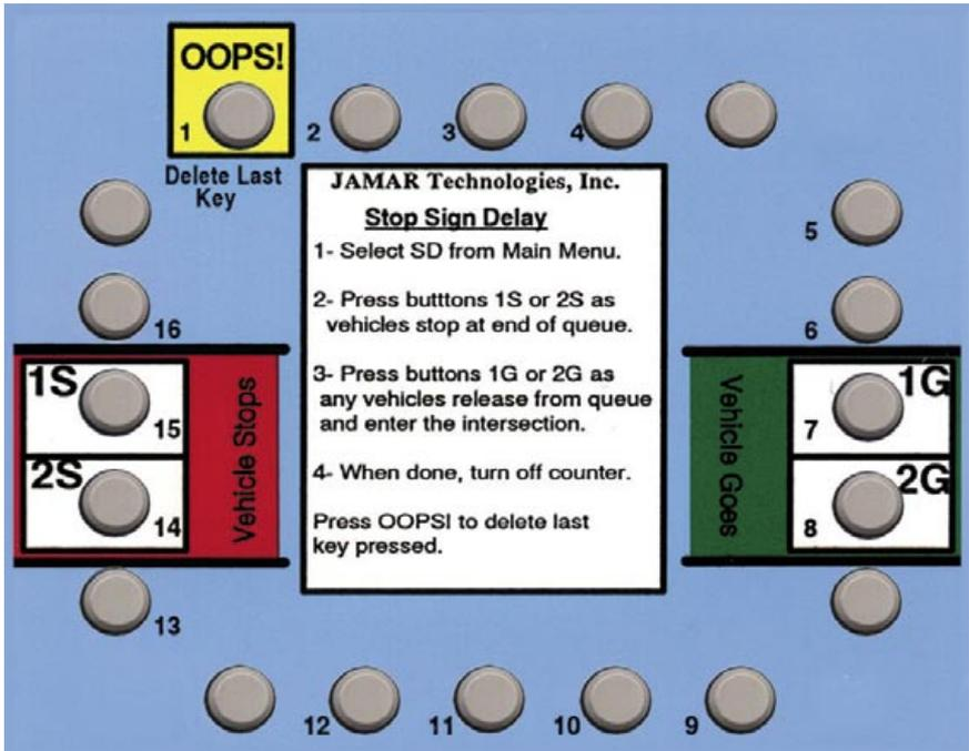
The Stop Sign Delay study in the TDC-12 is designed to allow you to measure the traffic characteristics at an intersection controlled by a stop sign. Although it primarily measures delay, it also provides information about the queue length and traffic volumes at an approach.
