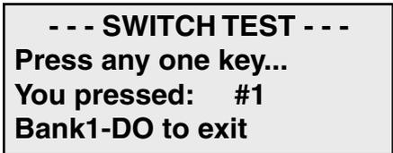
Each time you press a key, the TDC-12 displays the number of the key on the display. The BANK1, BANK2, TAB, & DO keys are spelled out. Press each of the keys until the all of the switches have been tested. Press BANK1 - DO to return to the TESTS menu.
