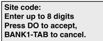
It is simple to enter the Site Code. Use the keys 1-10 like a keyboard (10=0). Enter the number you want. The display shows the numbers as you type them in. If you make a mistake, press BANK1-TAB and start over. When the number on the display is correct, press DO and you will go to the interval menu.
