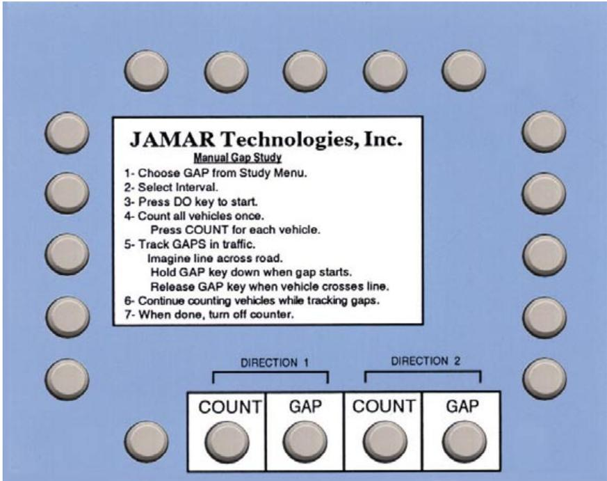
The TDC-12 makes it very simple to do manual gap studies. Most of traffic engineering is involved, one way or another, with managing gaps in traffic. After all, the primary purpose of a signal at an intersection is to artificially create gaps so that traffic can smoothly flow through an intersection. Even though gaps play an essential role in defining traffic patterns, there have been no instruments designed to help manually measure gaps, until the TDC-12.
