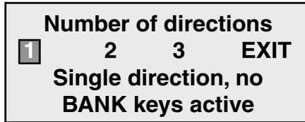
This screen allows you to decide how many directions of data to collect. If you select 2 or 3, while doing the study you use the BANK keys in conjunction with the primary 16 keys to record data for a second or third direction.
