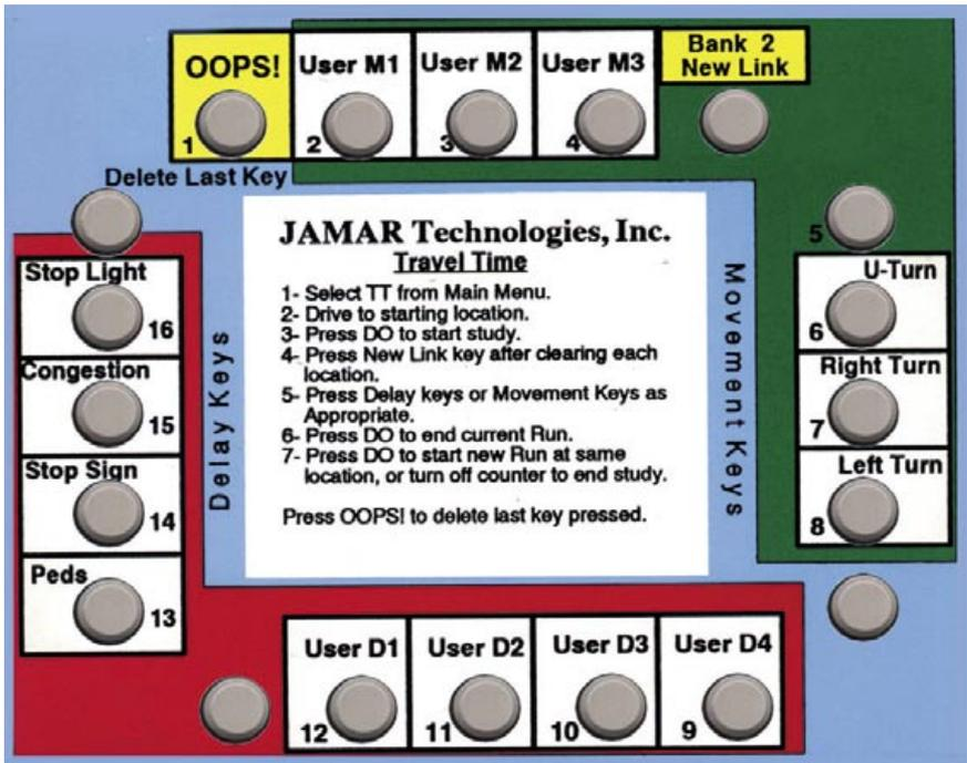
Travel Time data can be used to determine problem areas where significant delays are occurring and compare before and after data when changes have been made to signal timings.
