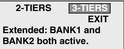
Press the TAB key to select the option you want, then press DO. The option is stored in memory, and you are returned to the Options menu. Note that if the 2-Tier mode is used, then the BANK 2 switch on the TDC-12 is disabled. You are then limited to 32 movements, with the primary movements counted with keys 1-16 and the secondary movements counted with the BANK1 key in conjunction with keys 1-16.
