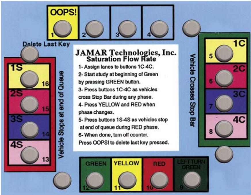
The Saturation Flow Rate study in the TDC-12 is actually a way to measure several separate but related traffic parameters. With one study you can measure:
