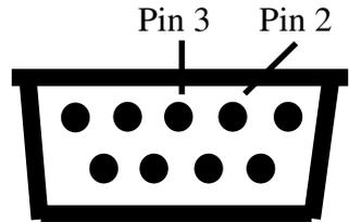
The TDC-12 sends a series of known messages out of the serial port, and at the same time reads the messages coming into the serial port. Since they are the same messages, the TDC-12 can tell if it is sending and receiving correctly. This tests the entire serial port section of the TDC-12 circuitry.
