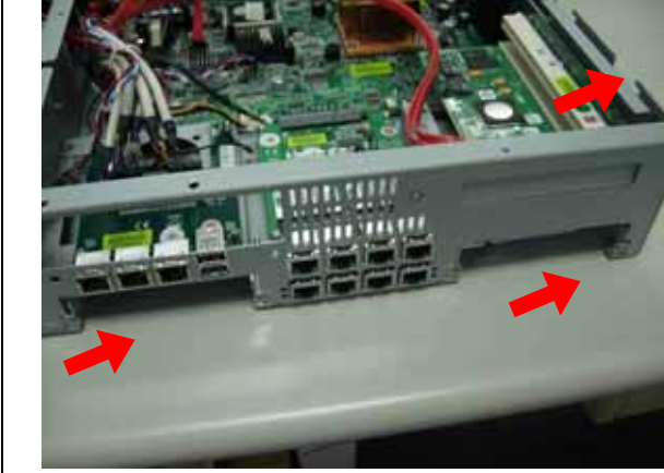
Fig.2-27 Remove all add-on modules.
