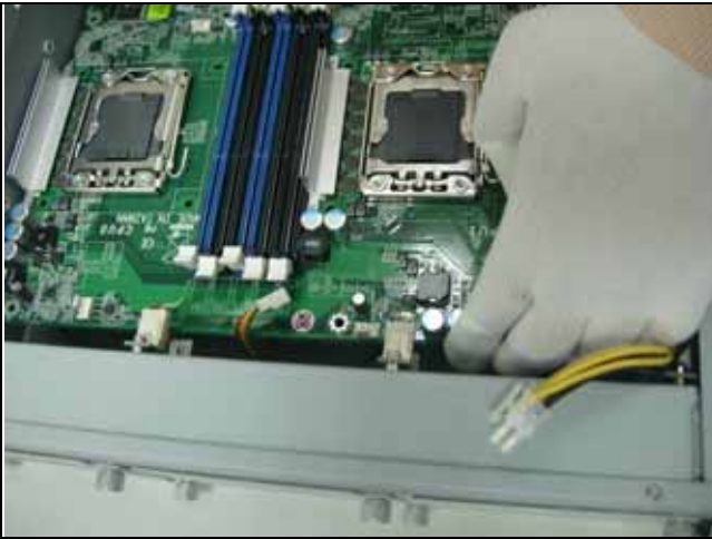
Fig.2-32 lift up main board from system from rear side.
