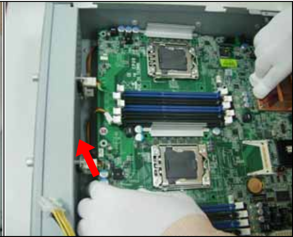
Fig.2-33 Lift the board up for moving.
