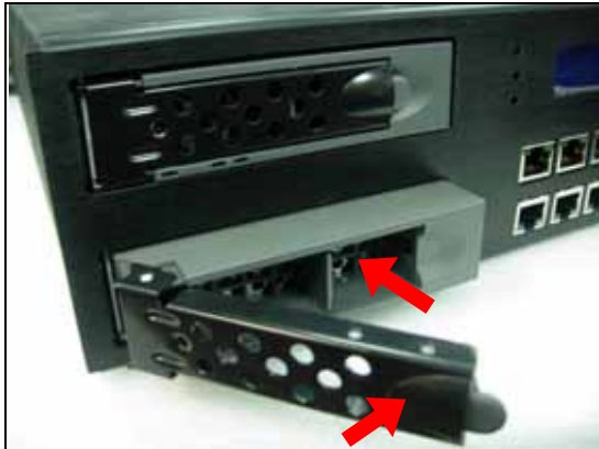
Fig. 2-12a Connect HDD bracket to NAR-7100 system then push the switch in.
