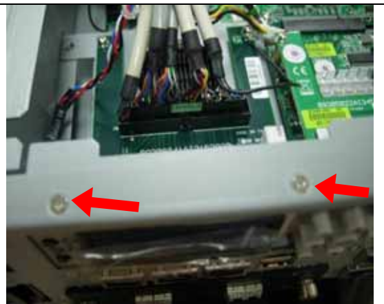
Fig.2-17 Remove screws from chassis.
