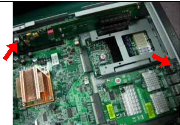
Fig. 2-11b Fix riser card to NAR-7100
