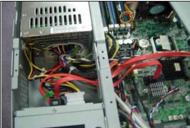
Fig.2-23 Remove all power cables from board and HDD bay.
