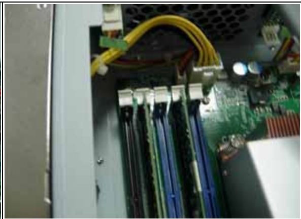
Fig.2-24 Remove all cables from board.
