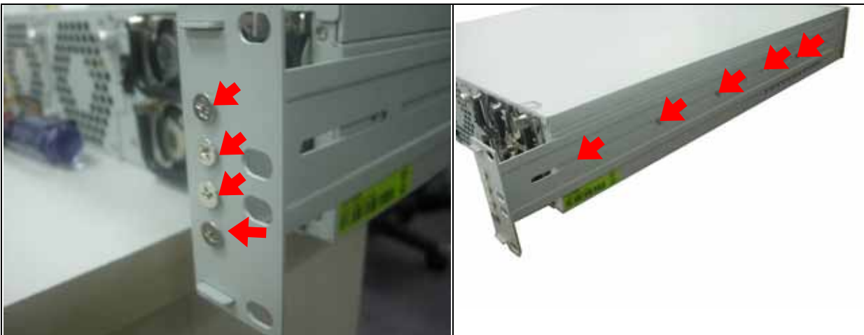
Fig.2-13.2 Fasten the screws to the side
