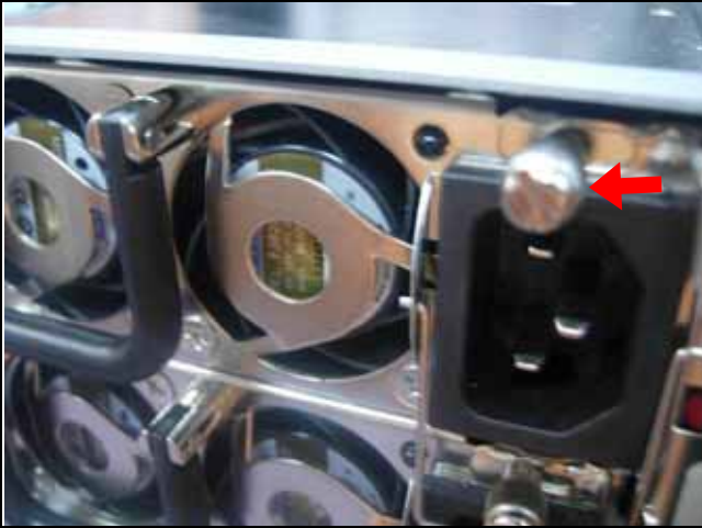
Fig.2-26.1 Loosen the screw to unlock the power module.
