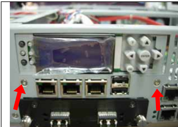
Fig.2-16 Remove the screws from EZIO
