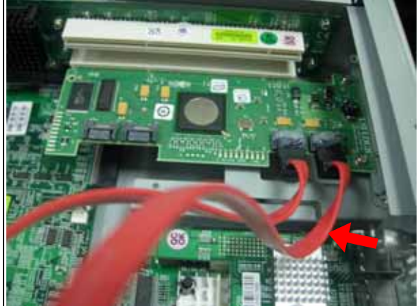
Fig.2-28 Remove riser card.
