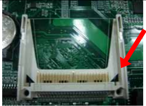
Fig. 2-7 Insert Compact Flash Card into the CF interface
