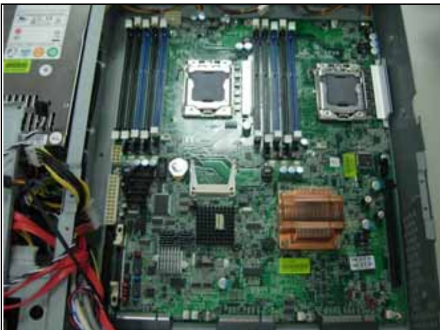
Fig.2-31 Remove all screws from main board.
