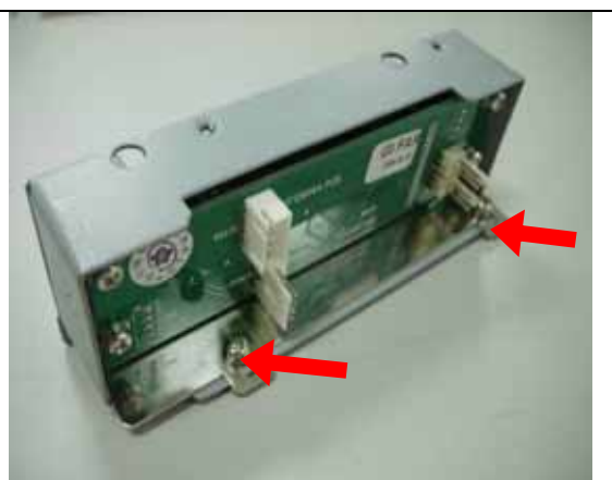
Fig.2-19 Remove the screws from EZIO kit
