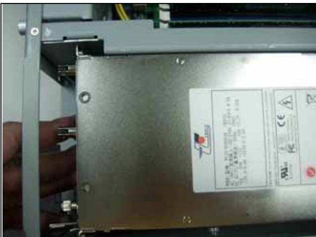
Fig.2-25.1 Push the power supply inside system.
