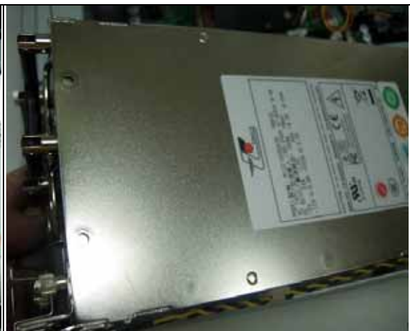
Fig.2-25.2 Pull out the power supply.
