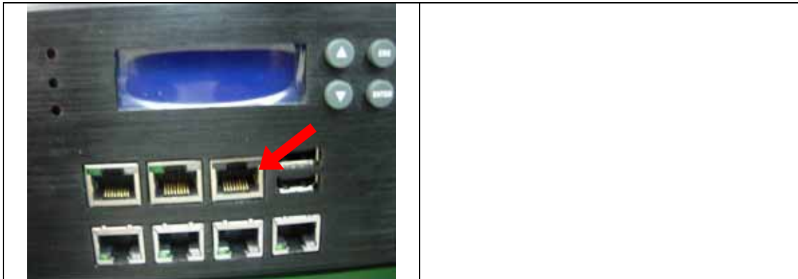
Fig.2-36 Connect null serial port cable to NAR-7100 console management port.
