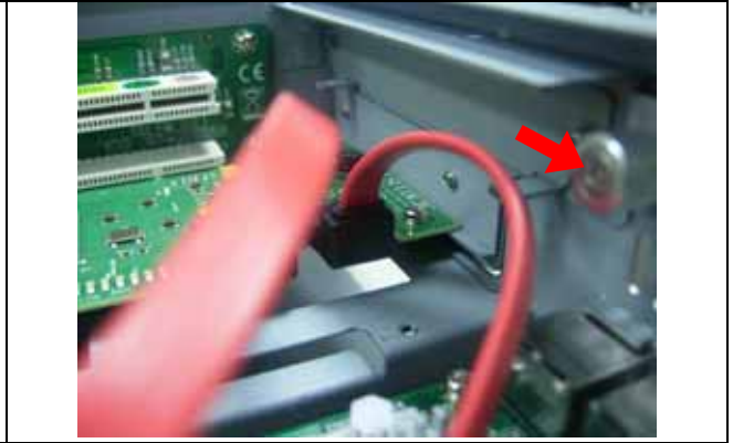
Fig. 2-11d Loosen the screw. Then unplug all SATA cables.
