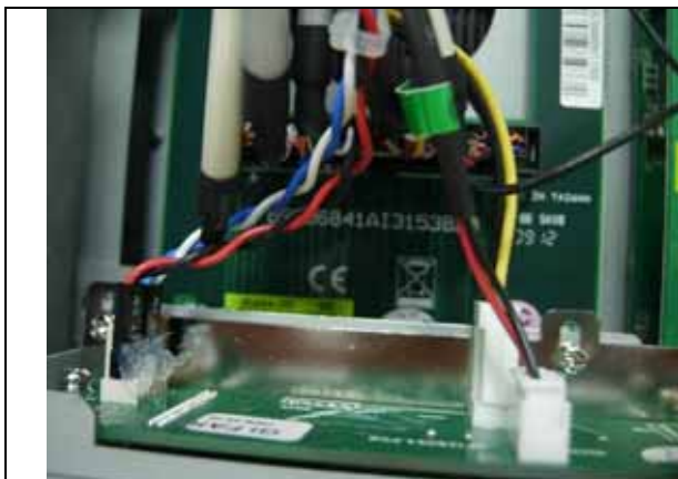
Fig.2-14 Remove the cable from EZIO
