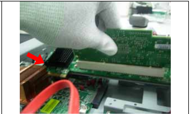
Fig. 2-11f Rotate the riser to proper angle to move out.
