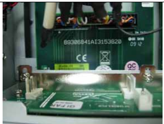
Fig.2-15 After remove the cable from EZIO
