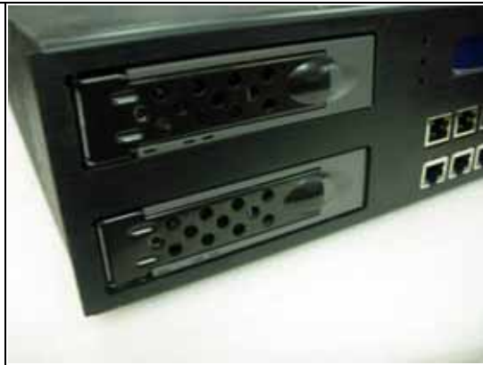
Fig. 2-12b Fix HDD into NAR-7100 system
