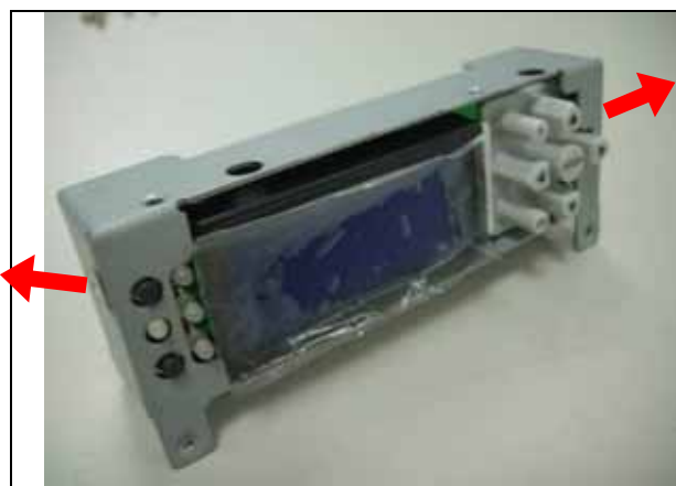
Fig.2-18 Remove the screws from EZIO kit
