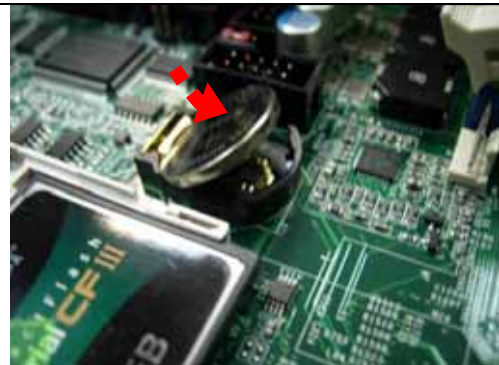
Fig. 2-10 Restore the battery
