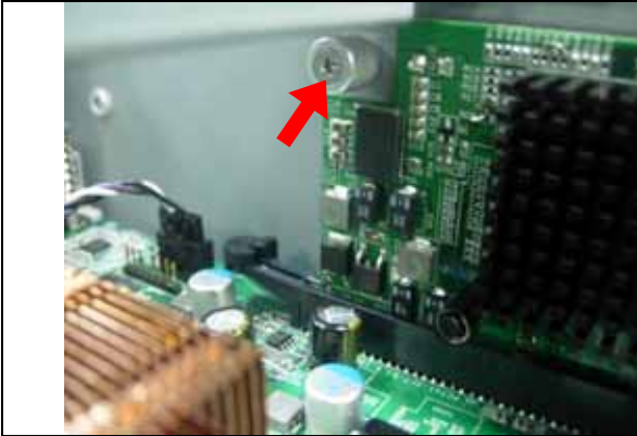
Fig. 2-11c Loosen the screw.
