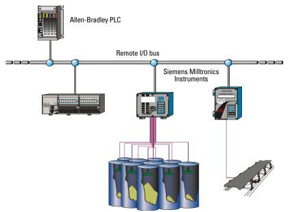
Remote I/O is an industry standard protocol owned by Allen-Bradley<sup>®</sup> which is part of Rockwell Automation. For a full description of the Remote I/O protocol, contact Rockwell or visit their web site at <u>www.rockwell.com</u>.
