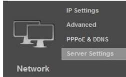
A “server” in this case is an Email account, FTP site or Samba network share, each of which must be configured in order to send or save notifications, snapshots or short video recordings. While all methods can be used, only Email is needed for notifications.
