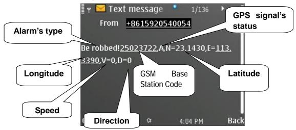
**Example**: The above message shows that: the SOS anti-robbery button is pressed down. The GSM base station code of the car is 25023722, the car is at outdoors & GPS signal is available, the latitude is 23.1430N, the longitude is 113.3390E, the car's speed
