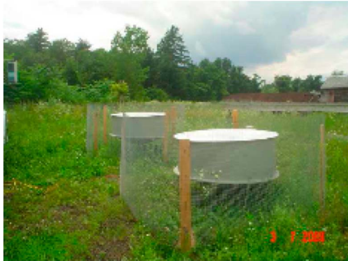
Figure 3.3: Shroud fence built around the Wind Profiler antennas
