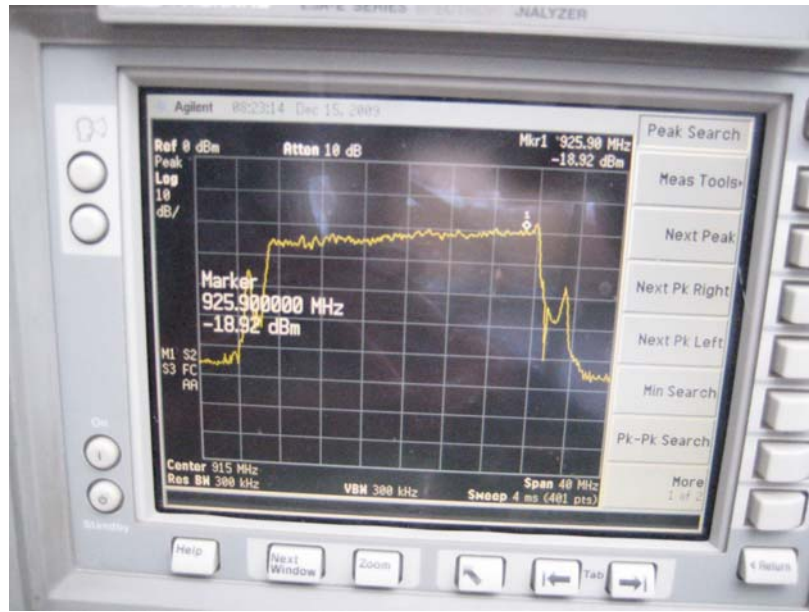
Figure 6.2: Received leakage without using shrouds
