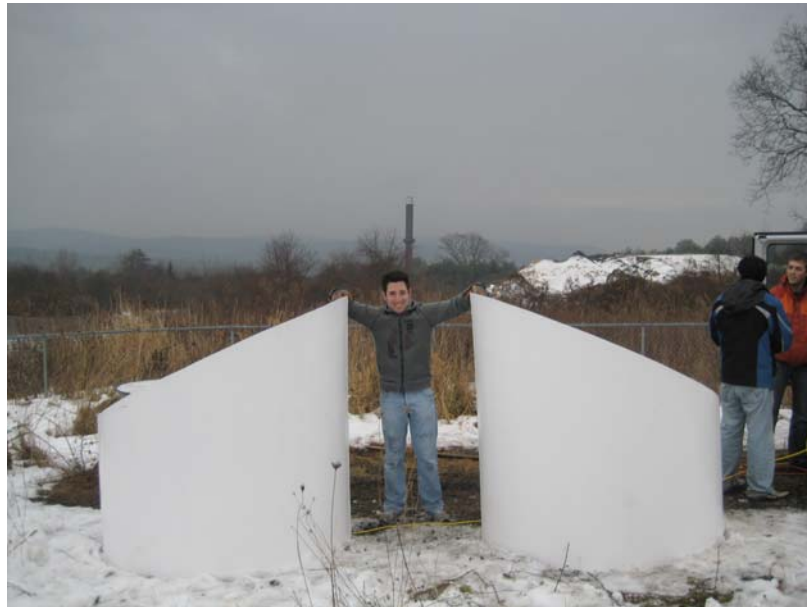
Figure 6.3: Wind Profiler deployment with shrouds
