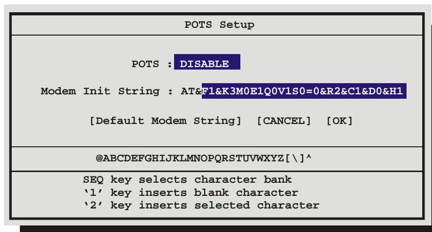
1. With the Modem Init String highlighted, press the **Enter** button to enter the Edit mode. The character bank will appear in the center of the menu.
