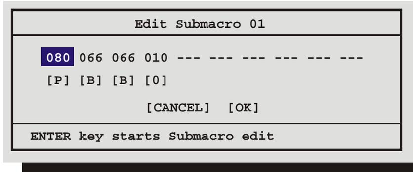
Use this menu to create the RS232 command string. Press the **Enter** button to Enter and Exit the submacro edit mode. Rotate the **Jog/Shuttle** to navigate among the fields and change the values. Each byte value can be set from 0 to 255.
