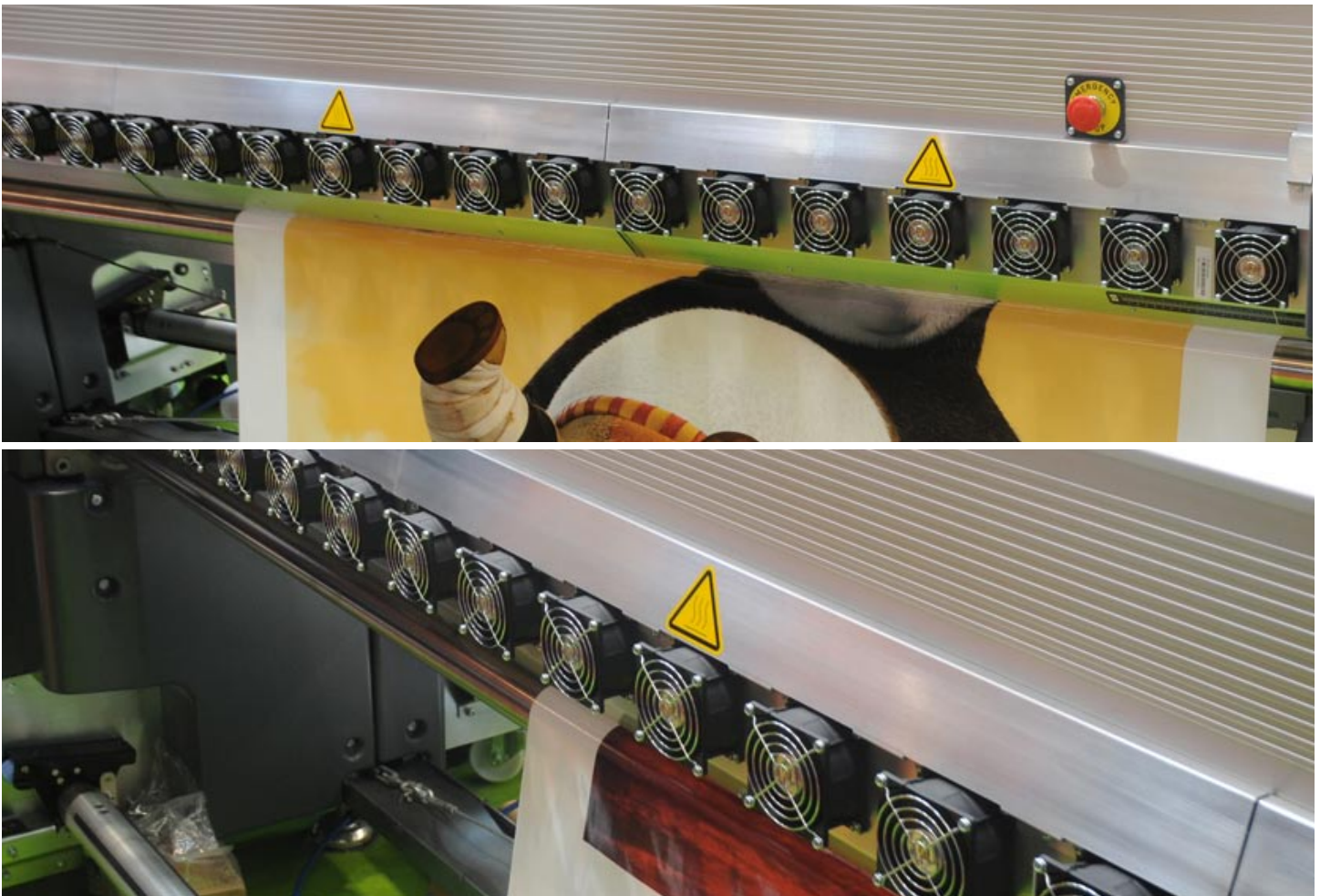
Fans on the HP Designjet L65500, photograph taken at FESPA Amsterdam, 2009.
