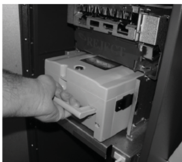
Removing note tray from the dispensing mechanism.
