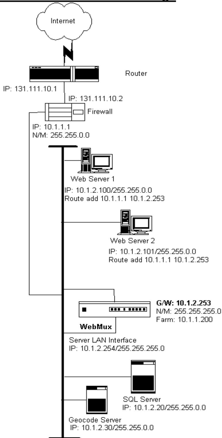
The above diagram is an example about how to install the WebMux without changing the IP addresses of the web servers and other servers that already
