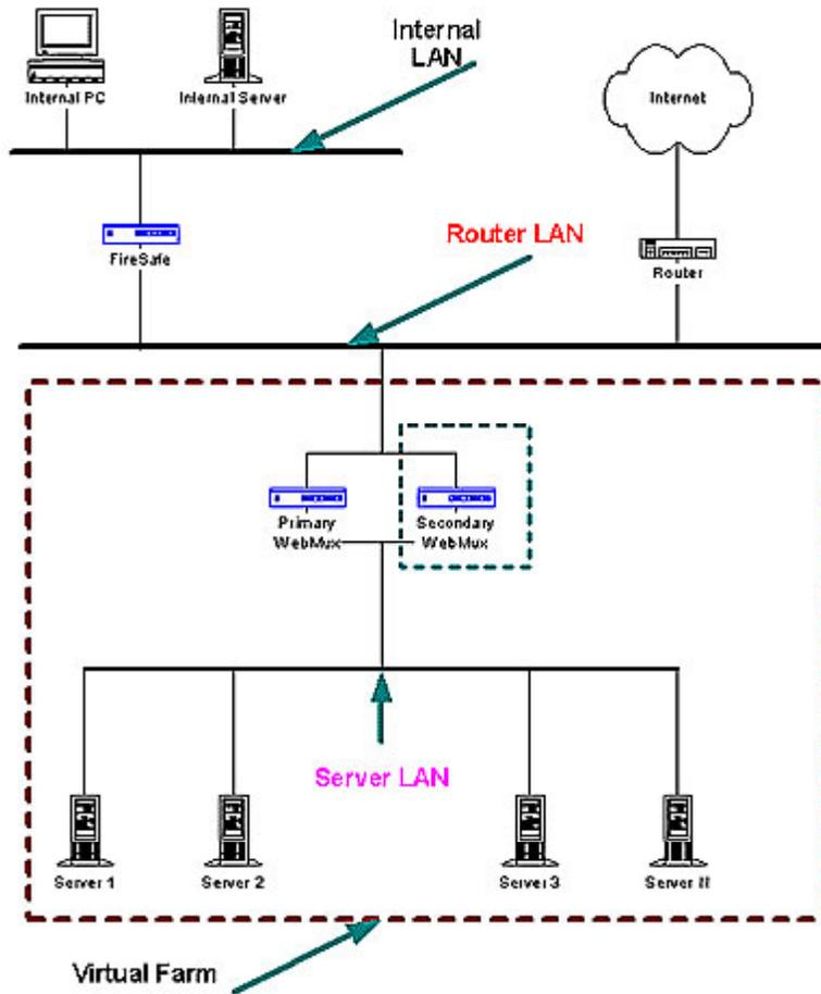
The main purpose of the WebMux is to balance the traffic among multiple web servers. The diagram above shows an installation with two WebMuxes. In this configuration, one WebMux serving as the primary, and the other serving as the secondary, or backup, provides a fault tolerant solution.
